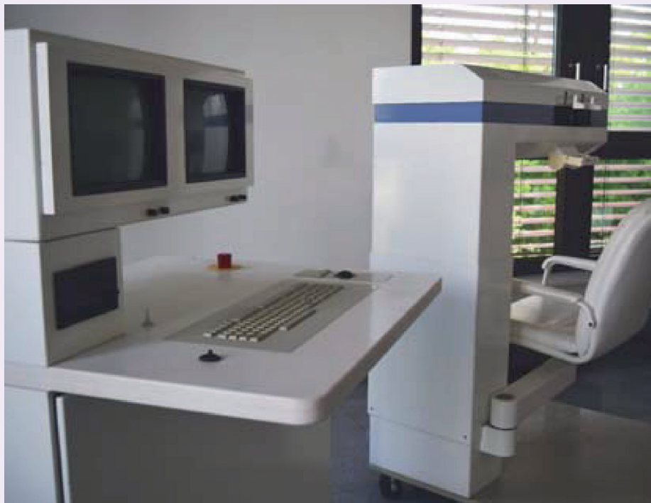
Figure 3. An early "massive, monstrous" retinal scanner.
